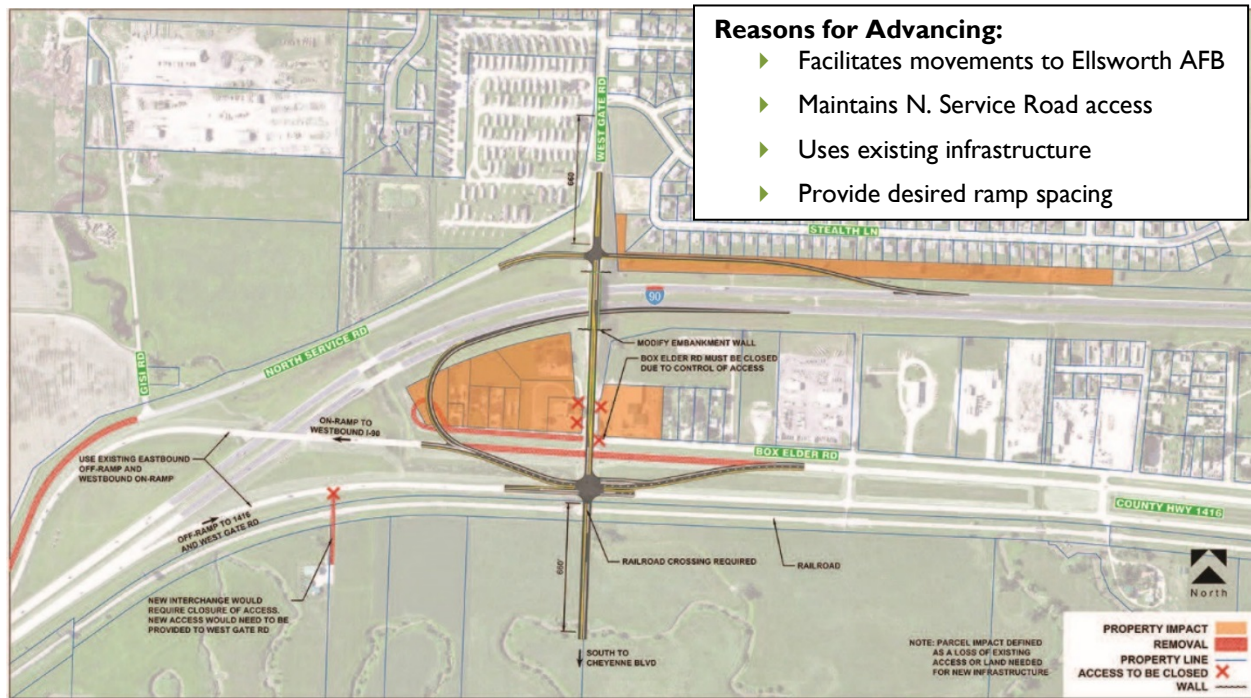
Figure 5-4. Alternative 3. Interchange at West Gate Road with Existing West Ramps and New East Ramps
