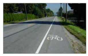
Figure 11. Shoulder bikeways are delineated with a fog line, and can use pavement stencils and signs.
