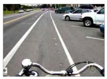
'Back-in' diagonal parking is safer for cyclists than 'head-in' diagonal parking due to drivers' visibility as they exit the parking spot.
