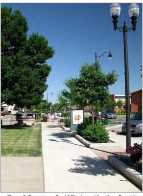
Figure 3. Downtown Rapid City has wide sidewalks with planters and pedestrian-scale lighting in the buffer zone.
