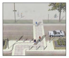
Figure 35. Mid-Block Pedestrian Crossing Concept.
