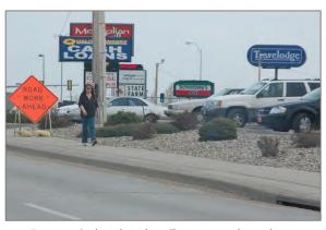
Figure 5. Curb-tight sidewalks on arterials can be an uncomfortable walking environment.
