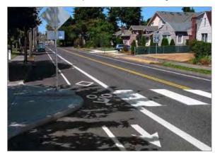
Figure 12. Designated bike lanes are designated with pavement markings and signs, and parking is prohibited.
