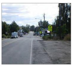
Roadway widening is preferred on roads lacking curbs, gutters and sidewalks.
